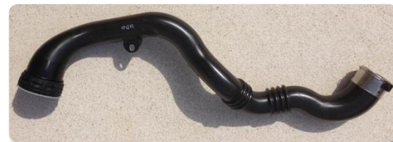
Arnitel HT in high temperature Airducts
